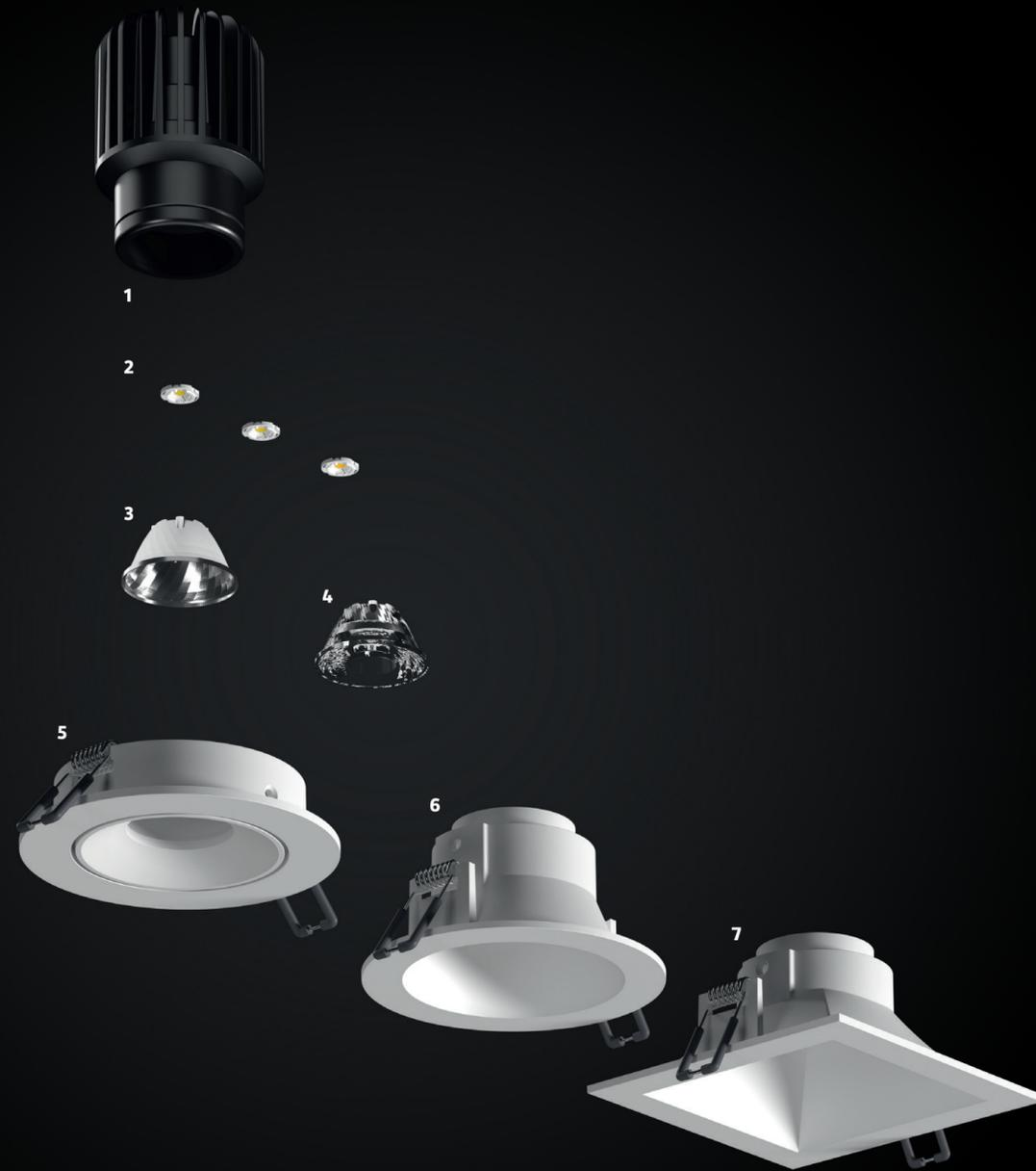
1 KÜHLKÖRPER 2 LED-PLATINE 4000 K, 3000 K, 2700 K 3 REFLEKTOR 4 LINSE 5 INNENRING BÜNDIG ABSCHLIESSEND, RUND 6 INNENRING ZURÜCKVERSETZT, RUND 7 INNENRING ZURÜCKVERSETZT, QUADRATISCH
